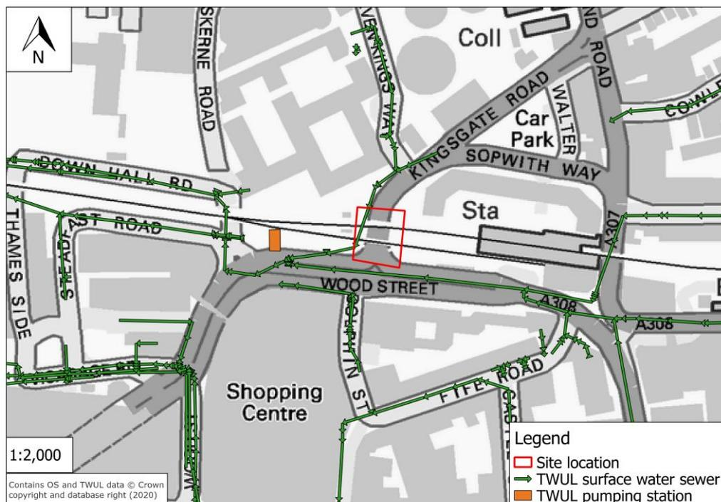
**Figure 3.4** TWUL surface water sewer system and pumping station
