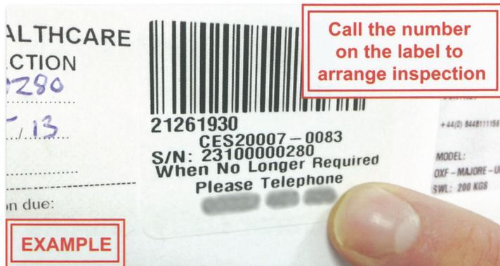
3. If SWL is not displayed or LOLER inspection is over six months old, DO NOT USE. Arrange inspection.
