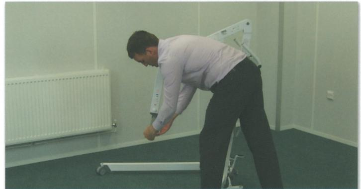
6. Ensure the spreader bar is firmly attached to the boom; and the boom is not damaged (bent or dented).
