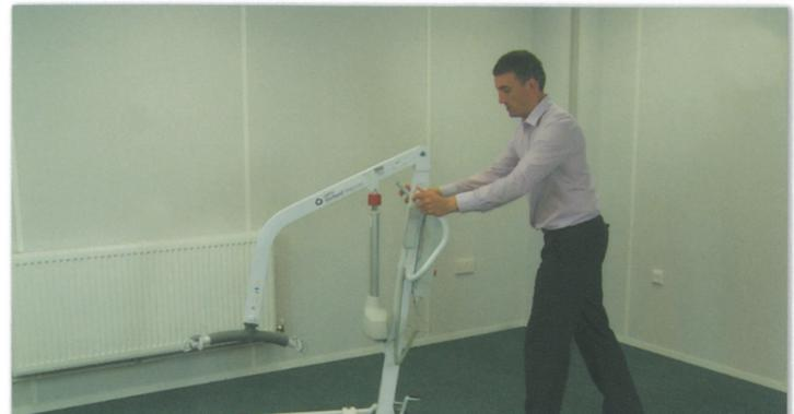
4. Check that hoist moves freely on its castors. Check the breaks on the castors work correctly.
