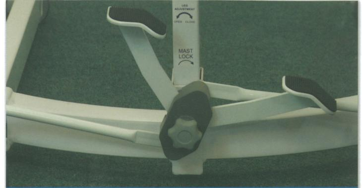
12. Ensure the mast stem fully engaged into the base. The locking knob fully tightened.
