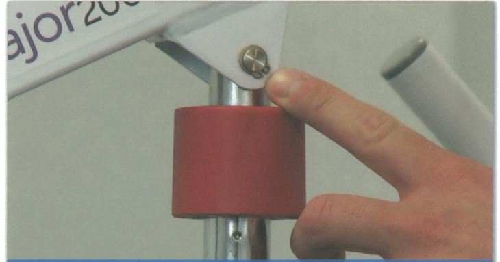
8. Check all fastenings on the actuator. Check the actuator for signs of damage.
