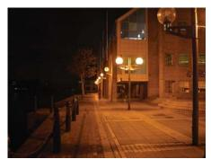
Distinct column and wall mounted luminaire family using sodium lighting.
