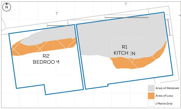
Figure 02: Example NSL diagram
