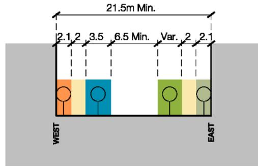
Figure 6.18: Street coding section: between Plot D and Plot G.
