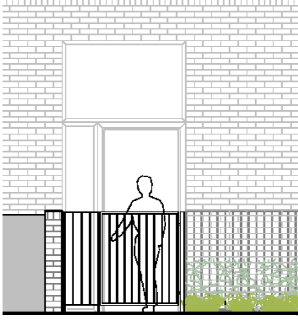
Figure 7.18: Typical entrance gate elevation
