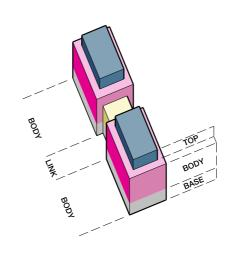
Figure 5.47: Terraced pairs must incorporate a recessive central linking piece.
