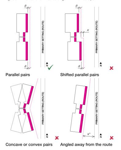
Figure 5.43: Terraced pairs must be aligned parallel to the route.
