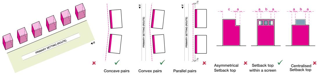
Figure 5.37: Pavilions positioned parallel to public route is prohibited.
