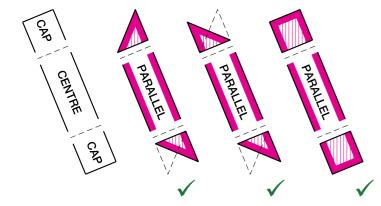
Figure 5.9: Plan diagram -Façades within the centre of building masses must be parallel.
