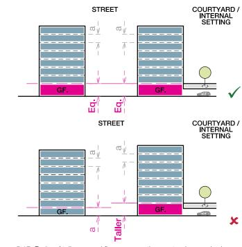
Figure 5.17: Parity of taller ground floors across the masterplan required.
