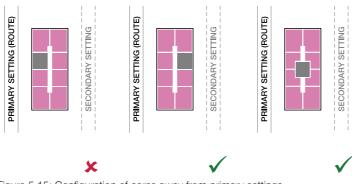
Figure 5.15: Configuration of cores away from primary settings.
