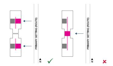
Figure 5.46: Separate entrances required to each building volume.
