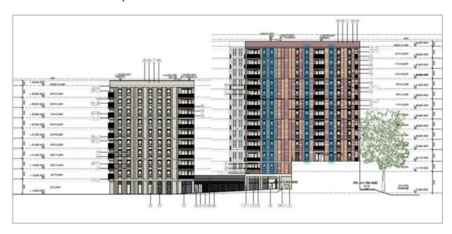
Figure T5.1. Block C1, east elevation. Windows that require blinds are marked up in blue (Patel Taylor drawings 23.10.2020).
