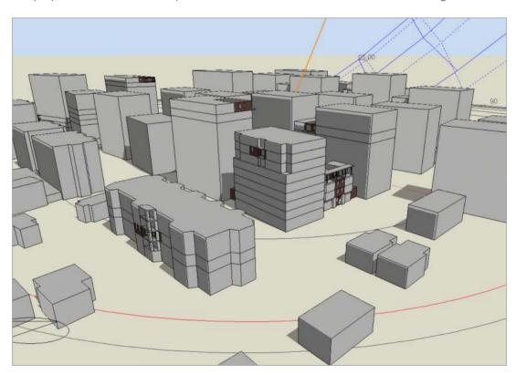
Figure 4: Design builder simulation model for Blocks B and E, sun path shown for 21st June 12:00 noon BST.
