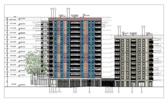
Figure T5.2. Block C1, west elevation. Windows that require blinds are marked up in blue (Patel Taylor drawings 23.10.2020).
