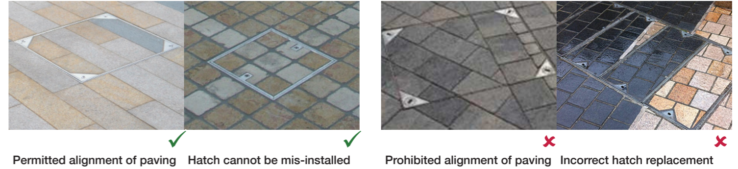
Figure 3.54: Inspection hatch Guidance.
