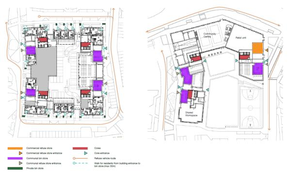
Figure 4: Refuse servicing diagram for Plot E [left] and Plot O [right] (Patel Taylor Architects, 2020)
