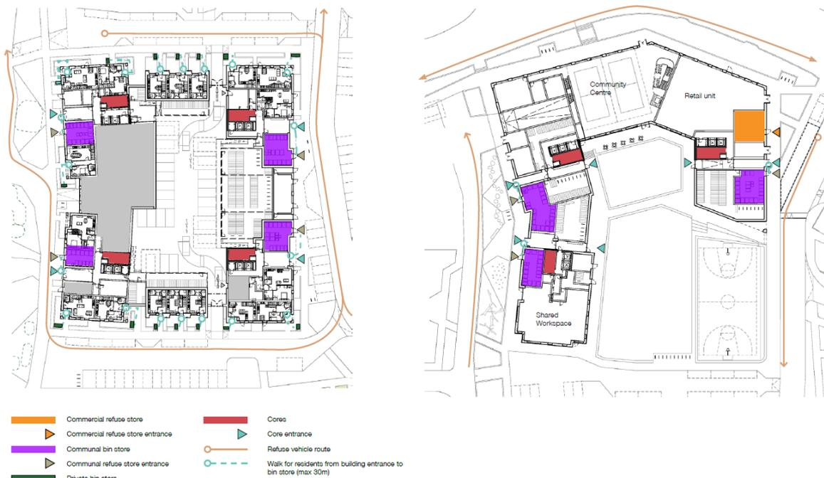
Figure 4: Refuse servicing diagram for Plot E [left] and Plot O [right] (Patel Taylor Architects, 2020)
