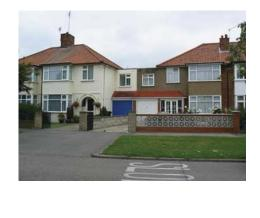
Figure 38 This is an acceptable first floor side extension where the gap between the two dwellings has been retained by setting the extension in from the shared boundary
